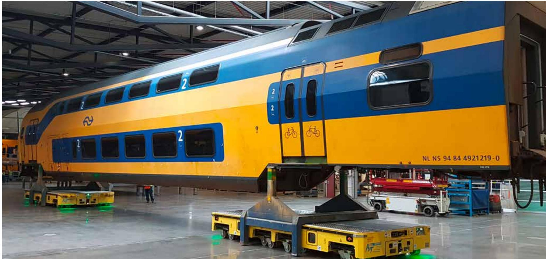
When coupled, both cars behave as one unit, which makes the drivability and user interface highly convenient. Each set is equipped with two wireless remote controls for manual and semi-automatic control. Each car can be used independently.
